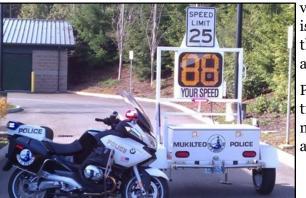
vehicles and displays the speed on a reader board. The goal is to heighten driver's awareness of both the speed at which they are traveling and the posted speed limit. This encourages drivers to adjust their speeds, if needed.
