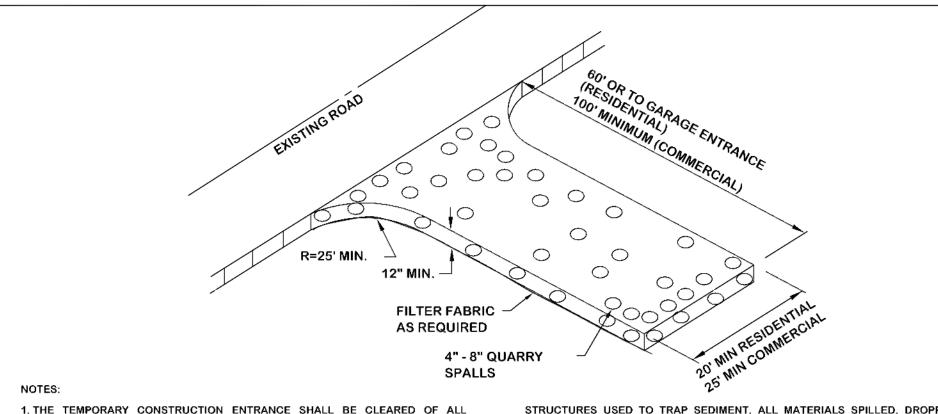
1. THE TEMPORARY CONSTRUCTION ENTRANCE SHALL BE CLEARED OF ALL VEGETATION, ROOTS, AND OTHER OBJECTIONABLE MATERIAL. ANY DRAINAGE FACILITIES REQUIRED BECAUSE OF WASHING SHOULD BE CONSTRUCTED ACCORDING TO SPECIFICATIONS IN THE PLAN. IF WASH RACKS ARE USED, THEY SHOULD BE INSTALLED ACCORDING TO MANUFACTURER'S SPECIFICATIONS.
