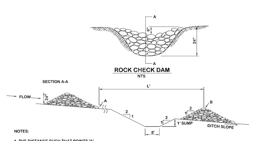
1. THE DISTANCE SUCH THAT POINTS 'A' AND 'B' ARE OF EQUAL ELEVATION.
