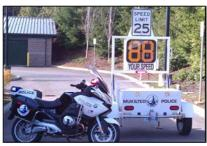
The radar trailer/dolly is a portable trailer equipped with a radar unit which detects the speed of passing vehicles and displays the speed on a reader board. The goal is to heighten driver's awareness of both the speed at which they are traveling and the posted speed limit. This encourages drivers to adjust their speeds, if needed.
