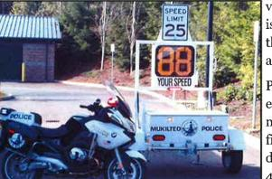
vehicles and displays the speed on a reader board. The goal is to heighten driver's awareness of both the speed at which they are traveling and the posted speed limit. This encourages drivers to adjust their speeds, if needed.
