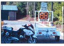
The radar trailer/dolly is a portable trailer equipped with a radar unit which detects the speed of passing vehicles and displays the speed on a reader board. The goal is to heighten driver's awareness of both the speed at which they are traveling and the posted speed limit. This encourages drivers to adjust their speeds, if needed.
