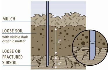
A rod penetrometer is a 4 foot long, 3/8 inch or 10 mm diameter stainless steel rod with a 90 degree bend 5 inches form the top to make a handle, and a 30 degree bevel cut 1/8 inch or 3 mm into the side of the tip.
