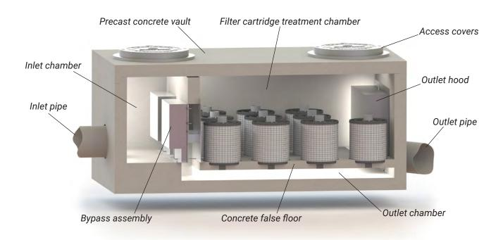
Figure 1. Schematic of the PerkFilter System.
