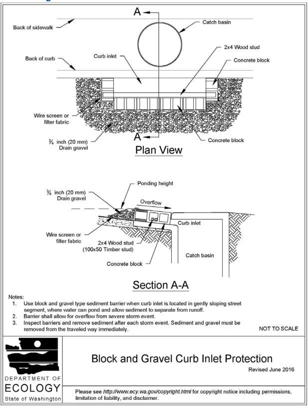
Figure II-3.18: Block and Gravel Curb Inlet Protection
