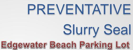
Thin mixture of emulsified asphalt, water & fine aggregate applied to road surface.
