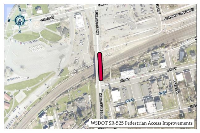
Pedestrian and Access Improvements, including widening the existing SR 525 bridge eastern sidewalk, re-configuring the existing lanes, and upgrade curb ramps to meet current ADA standards.
