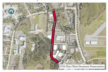
Extend the life of the pavement on 47th PI W by completing pavement grinding, HMA overlay, full depth pavement repair where needed, curb ramp upgrades to comply with ADA requirements, restriping, and upgraded signage to comply with MUTCD standards. Channelization may also be modified to include bicycle lanes, following an evaluation to determine community desire for this change.
