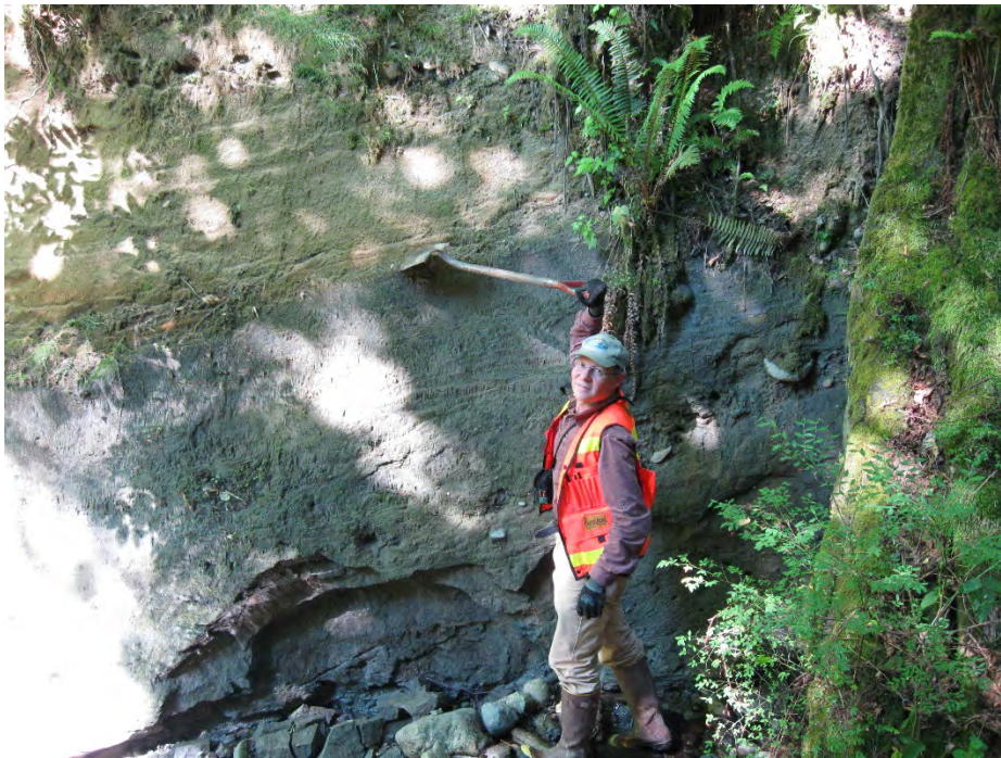
Photo #17. Contact between Vashon advance outwash (Qva) (top, light brown) and Transitional beds (Qtb) lacustrine deposits (bottom, gray).
