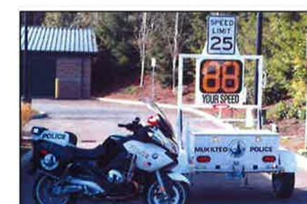
The radar trailer/dolly is a portable trailer equipped with a radar unit which detects the speed of passing vehicles and displays the speed on a reader board. The goal is to heighten driver's awareness of both the speed at which they are traveling and the posted speed limit. This encourages drivers to adjust their speeds, if needed.
