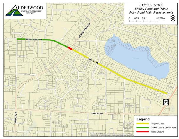
Sewer main line installation along Picnic Point Road from 52<sup>nd</sup> Ave W to Beverly Park Road is complete. In July and August, crews will install sewer laterals connecting the new main to private individual side sewers.
