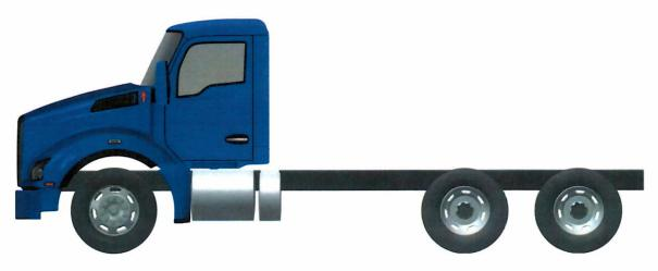
Recommended payload center of gravity to achieve specified ground loads; measured from centerline of drive axles: 24 in. from the centerline of the drive axle(s).
